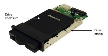
**Step 1:** Connect a SATA cable to the 7-pin SATA data connector to the SATA interface of the cradle.
